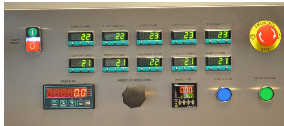
Control panel showing ten temperature controllers, plus digital pressure and digital dwell time controllers.
